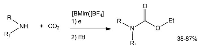
Fig. 15 Production of carbamates from the electroreduction of \text{CO}_2 in the ionic liquid [\text{BMIM}][\text{BF}_4] .
