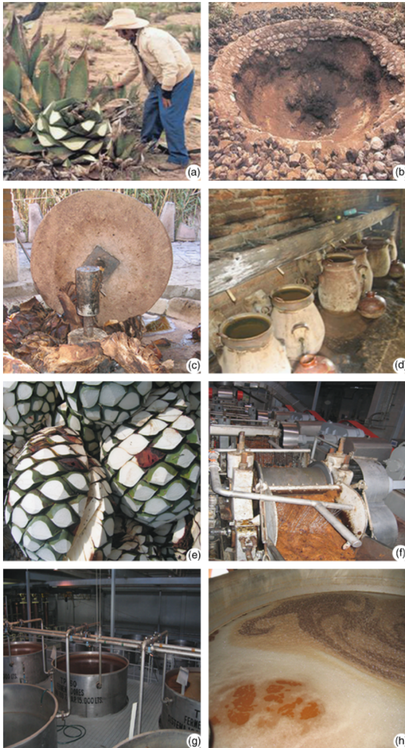
Fig. 2. Mezcal traditional and tequila industrial elaboration processes. (a) Agave pine of Agave sp. (b) Rustic ground oven. (c) Stone mill or tahona. (d) Clay pot stills. (e) Pines of Agave tequilana Weber var. azul . (f) Extraction of Agave juice in industrial mill. (g) Stainless steel industrial fermentation tanks. (h) Detail of the fermenting must.
